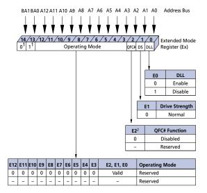
NOTE: 1. E14 and E13 (BA0 and BA1) must be "0, 1" to select the Extended Mode Register (vs. the base Mode Register).
