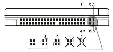
Figure 4 : Drive address setting
