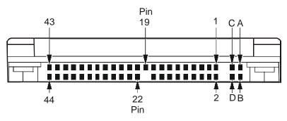
Figure 3 : Interface connector pin assignments
