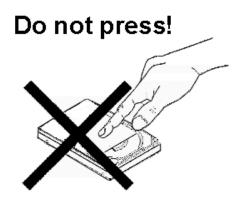
Do not press on the drive cover during handling.
