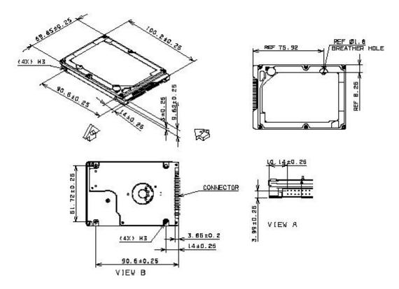
Figure 2: Mounting hole locations
