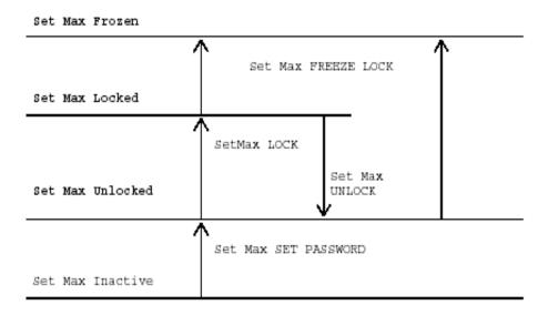
Figure 8: Set Max security mode transition
